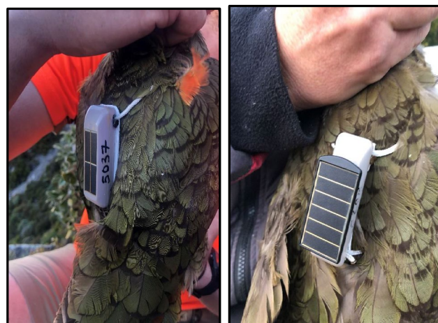
Figure 2. Images of Druid Debut Lego™ GPS trackers with a flush (left) and raised (right) solar panels on kea.
