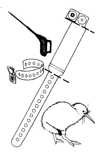
FIGURE 1- The new radio-tagging system for young kiwi showing the transmitter package (top left), the bracelet (middle diagonal), the two parts of the bracelet used to make the strap (middle left), and the transmitter in place (bottom right). The transmitter and bracelet are shown in actual size.
